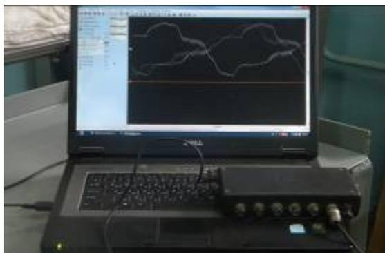
**Fig. 2. Computer oscillograph USB Oscilloscope for determining the contact difference of potentials**
