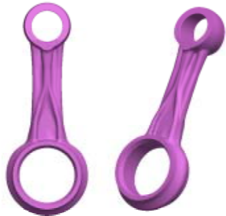
Fig. 3. New model of connecting rod after optimization
