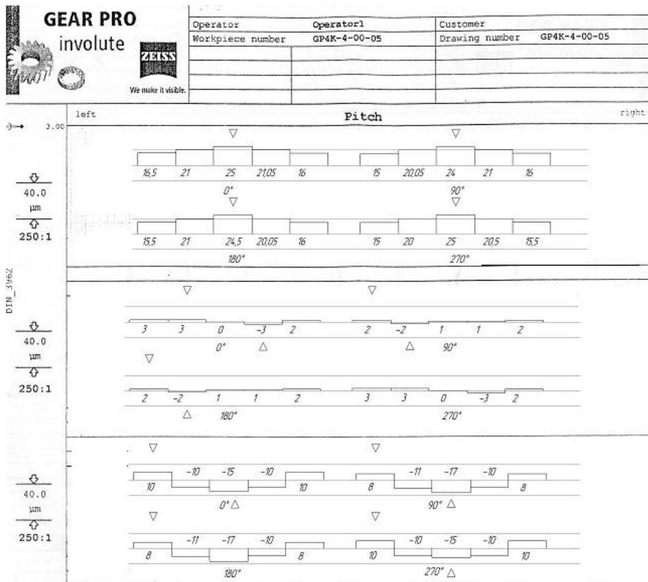
Figure 3. Protocol of measuring the outer cylindrical contour of the elastic helical hone on the coordinate measuring machine
