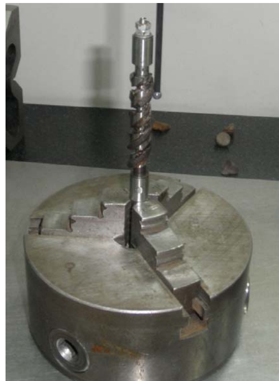
1 – Carl Zeiss CONTURA G2 coordinate measuring machine; 2 – measuring probe; 3 – elastic helical hone. a) a general view of the area of measurement of the outer cylindrical contour of the elastic helical hone; b) the area of measurement of the outer cylindrical contour of the elastic helical hone
