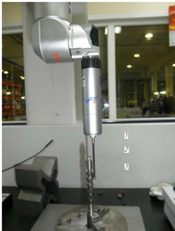
1 – Carl Zeiss CONTURA G2 coordinate measuring machine; 2 – measuring probe; 3 – elastic helical hone. a) a general view of the area of measurement of the outer cylindrical contour of the elastic helical hone; b) the area of measurement of the outer cylindrical contour of the elastic helical hone
