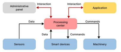
Fig. 2. Functional Diagram of the IoT Platform
