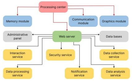
Fig. 1. Processing center architecture
