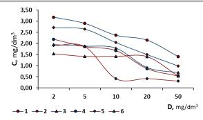
Figure 5. Change in the concentration of oil in fresh (1, 2, 3) and salt (4, 5, 6) water ([H<sub>initial</sub>]= 100 mg/dm<sup>3</sup>) depending on the dose of Al<sub>2</sub>(SO<sub>4</sub>)<sub>3</sub> (in terms of Al<sub>2</sub>O<sub>3</sub>) and the working concentration of the sorbent: 0 mg/dm<sup>3</sup> (1, 4), 50 mg/dm<sup>3</sup> (2,5), 100 mg/dm<sup>3</sup> (3, 6)
