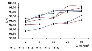
Figure 3. Dependence of oil removal from fresh (1, 2, 3) and salt (4, 5, 6) water ([H<sub>initial</sub>]= 100 mg/dm<sup>3</sup>) depending on the type of coagulant Al<sub>2</sub>(SO<sub>4</sub>)<sub>3</sub> (1, 4), Al(OH)<sub>3</sub> (2, 5), Al(OH)<sub>2</sub>Cl (3, 6), and their doses ( in terms of Al<sub>2</sub>O<sub>3</sub>)
