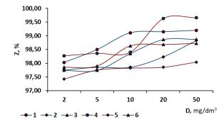
Figure 8. Dependence of oil removal from fresh (1, 2, 3) and salt (4, 5, 6) water ([H<sub>initial</sub>]= 100 mg/dm<sup>3</sup>) depending on the dose of Al(OH)<sub>3</sub> (in terms of Al<sub>2</sub>O<sub>3</sub>) and the working concentration of the sorbent: 0 mg/dm<sup>3</sup> (1, 4), 50 mg/dm<sup>3</sup> (2,5), 100 mg/dm<sup>3</sup> (3, 6)
