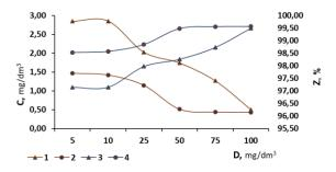
Figure 4. Dependence of residual oil concentration in fresh (1, 2, 3) and salt (4, 5, 6) water ([H<sub>initial</sub>]= 100 mg/dm<sup>3</sup> and degree of oil removal from fresh (3) and salt (4) waters on the sorbent dose
