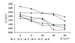
Figure 2. Change in the concentration of oil in fresh (1, 2, 3) and salt (4, 5, 6) water ([H<sub>initial</sub>]= 100 mg/dm<sup>3</sup>) depending on the type of coagulant Al<sub>2</sub>(SO<sub>4</sub>)<sub>3</sub> (1, 4), Al(OH)<sub>3</sub> (2, 5), Al(OH)<sub>2</sub>Cl (3, 6), and their doses (in terms of Al<sub>2</sub>O<sub>3</sub>)
