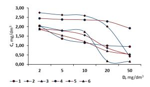
Figure 9. Change in the concentration of oil in fresh (1, 2, 3) and salt (4, 5, 6) water ([H<sub>initial</sub>]= 100 mg/dm<sup>3</sup>) depending on the dose of Al(OH)<sub>2</sub>Cl (in terms of Al<sub>2</sub>O<sub>3</sub>) and the working concentration of the sorbent: 0 mg/dm<sup>3</sup> (1, 4), 50 mg/dm<sup>3</sup> (2,5), 100 mg/dm<sup>3</sup> (3, 6)
