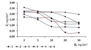
Figure 7. Change in the concentration of oil in fresh (1, 2, 3) and salt (4, 5, 6) water ([H<sub>initial</sub>]= 100 mg/dm<sup>3</sup>) depending on the dose of Al(OH)<sub>3</sub> (in terms of Al<sub>2</sub>O<sub>3</sub>) and the working concentration of the sorbent: 0 mg/dm<sup>3</sup> (1, 4), 50 mg/dm<sup>3</sup> (2,5), 100 mg/dm<sup>3</sup> (3, 6)
