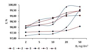
Figure 10. Dependence of oil removal from fresh (1, 2, 3) and salt (4, 5, 6) water ( $[H_{initial}]$  = 100 mg/dm<sup>3</sup>) depending on the dose of Al(OH)<sub>2</sub>Cl (in terms of Al<sub>2</sub>O<sub>3</sub>) and the working concentration of the sorbent: 0 mg/dm<sup>3</sup> (1, 4), 50 mg/dm<sup>3</sup> (2,5), 100 mg/dm<sup>3</sup> (3, 6)
