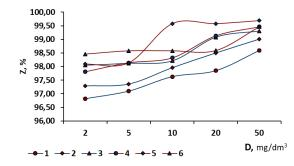
Figure 6. Dependence of oil removal from fresh (1, 2, 3) and salt (4, 5, 6) water ( $[H_{initial}]$ = 100 mg/dm<sup>3</sup>) depending on the dose of Al<sub>2</sub>(SO<sub>4</sub>)<sub>3</sub> (in terms of Al<sub>2</sub>O<sub>3</sub>) and the working concentration of the sorbent: 0 mg/dm<sup>3</sup> (1, 4), 50 mg/dm<sup>3</sup> (2,5), 100 mg/dm<sup>3</sup> (3, 6)
